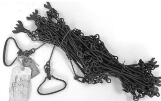
Chain measure used to measure out the Oxpens allotments, early 20thc. Donated by Nick Potter, bought at Kearsley's farm sale
